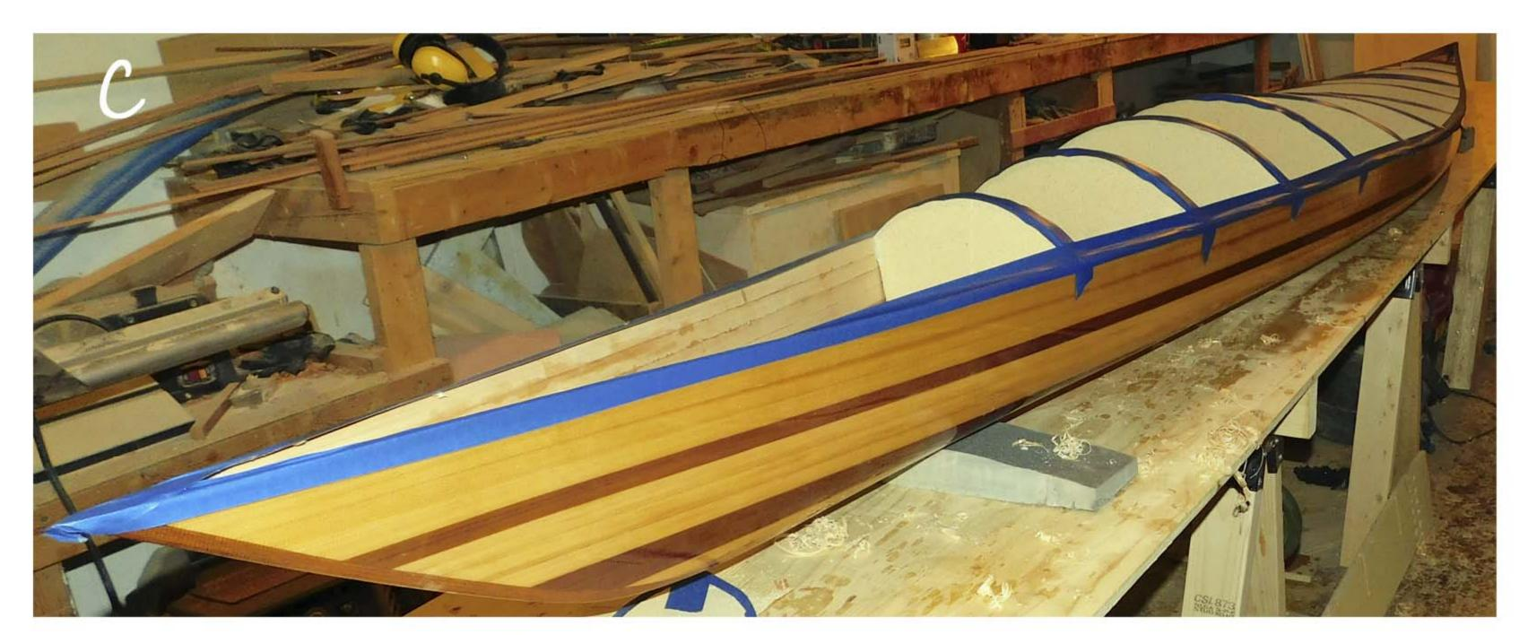
Shown above is a rapid start set up for the Pukaskwa 15 kayak. Kayak systems are set up to allow for the construction of the hull then the hull is flipped and the same molds are trimmed to facilitate construction of the deck.
