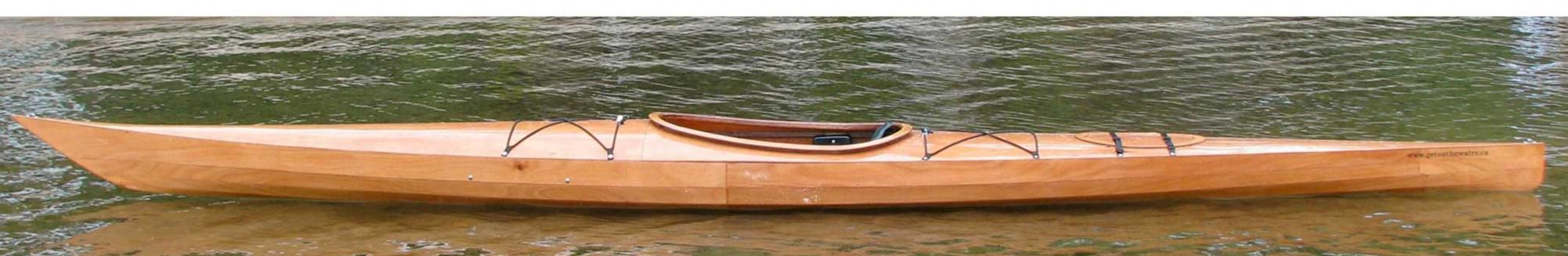
Length 17 ft. 5.18 m. Beam 23 in. 58.4 cm Beam Waterline 22 in. 56 cm. Weight 40 lbs. 18 kg. Cockpit Depth 11 in. 28 cm. Recommended Load Range 150 to 230 lbs. 68 to 105 kg. Maximum Capacity 315 lbs. 143 kg.
