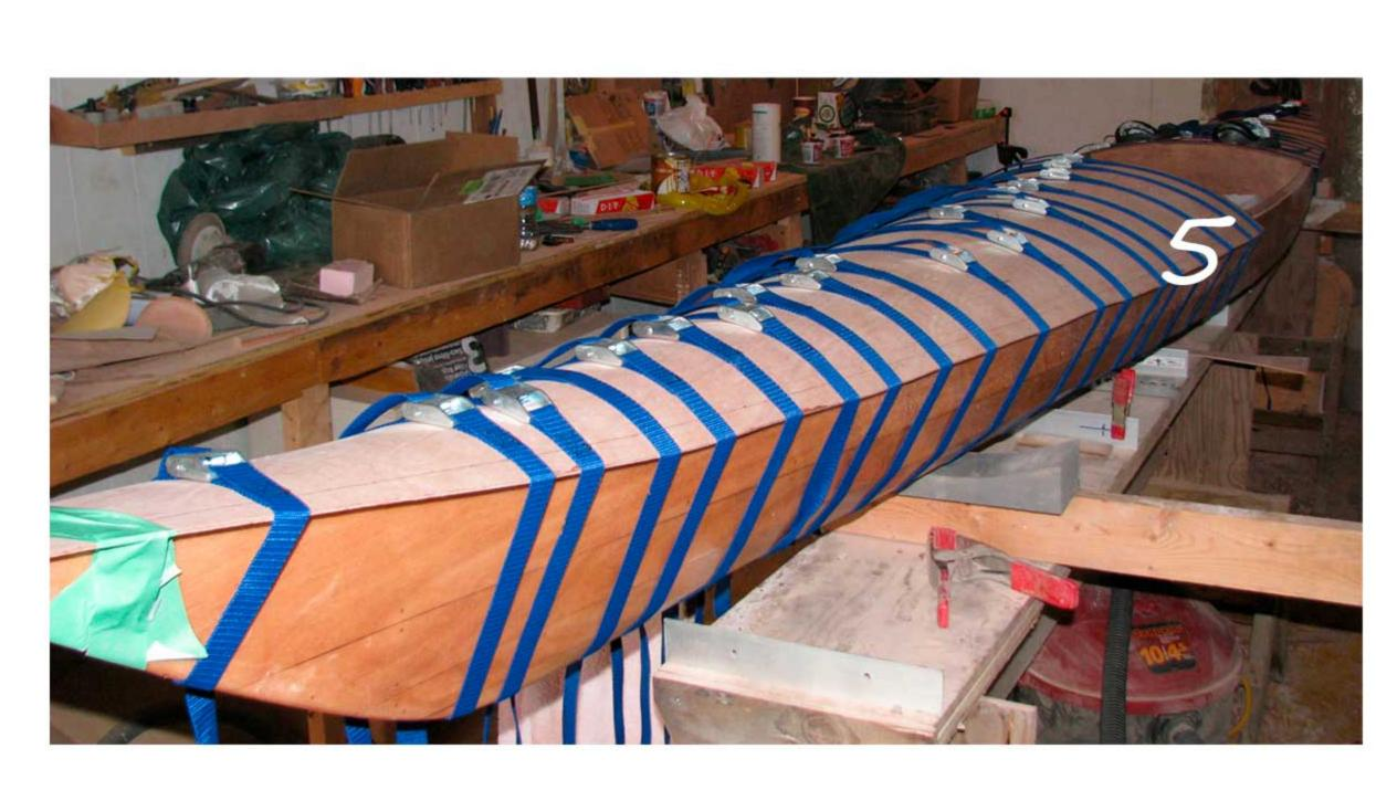
The Sport 17 is a multi chine, easily paddled boat, it is available with either a plywood deck as pictured or as a hybrid with a cedar strip deck. In the case of a cedar strip deck, the three larger panels at the bottom of the plywood kit parts drawing are replaced with a set of cedar strips and some additional fiberglass to sheath the cedar with.
