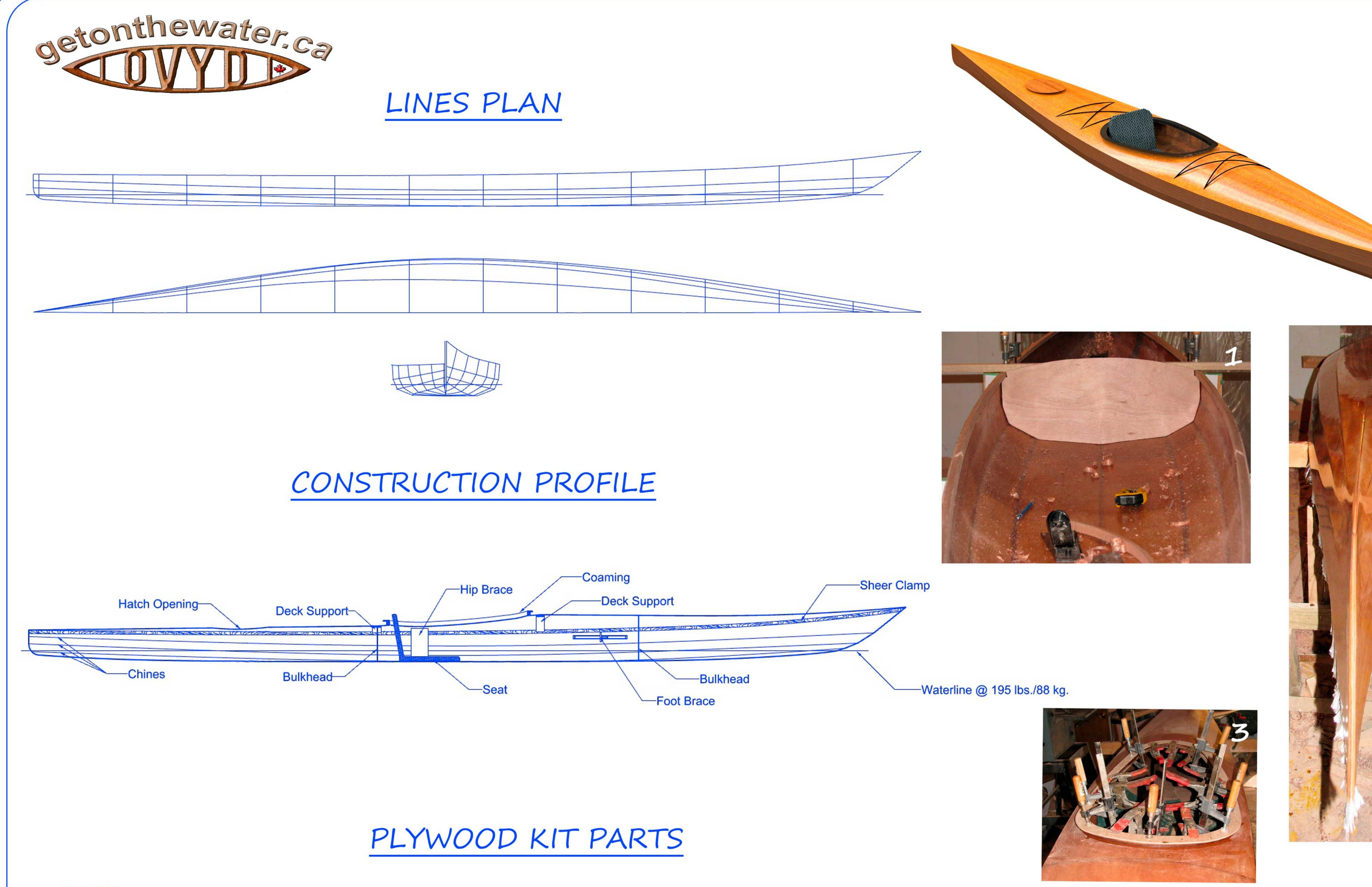
A wider version of the 17 originally developed for a client in France, like the others in this series it has a multi chine hull and can be constructed with either a plywood or a cedar strip deck. The extra beam gives more initial stabilty as well as increased capacity. Pictures are from the standard version as the build is the same and we have not had the opportunity to build one here at the shop.
