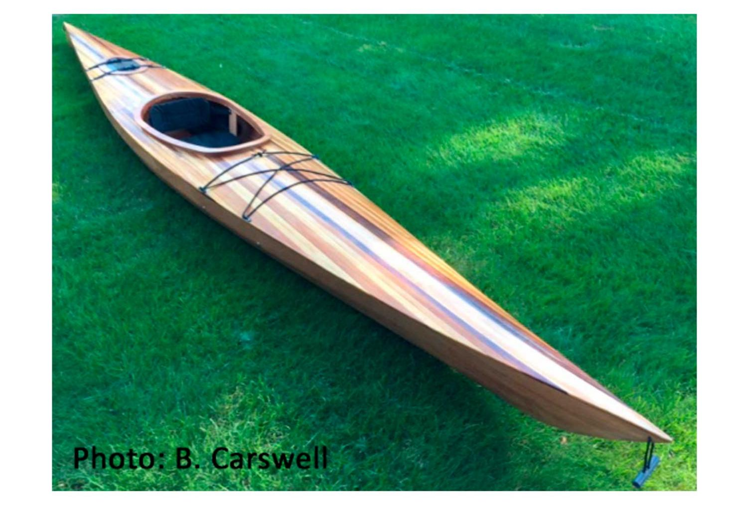
Photo shows a hybrid version of the 15. The boat is designed as a recreational kayak fetauring an easily paddled multi chine hull. Boats can be built from kits or from scratch.
