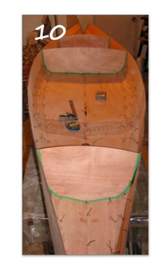
The pictures to the left illustrate the beginnings of a stitch and glue build, once you reach the point where the parts are made and are assembling the panels, the process is the same whether you are building from a kit or from scratch.
