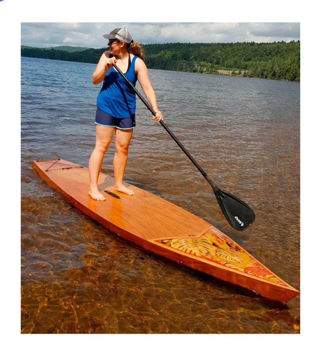
Paddle boards are available only as kits which have been designed to be as easy to assemble as possible. The main structure nterlocks and is assembled on a flat surface, this same base then is used to mount the jigs that guide the assembly of and joining of the hull and structure. The fin on this boat is fixed to the hull.
