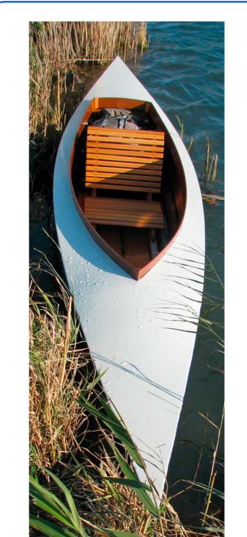
Designed as a tripping boat using the efficient hull of a kayak with easily packable hull of a canoe. These boats are suitable for anyone who wants or needs to carry cargo whether it is camping gear, children or pets. With the adjustable seat the boat can be kept level under numerous load conditions. There are a number of seating options for the builder, and optional cockpit covers.
