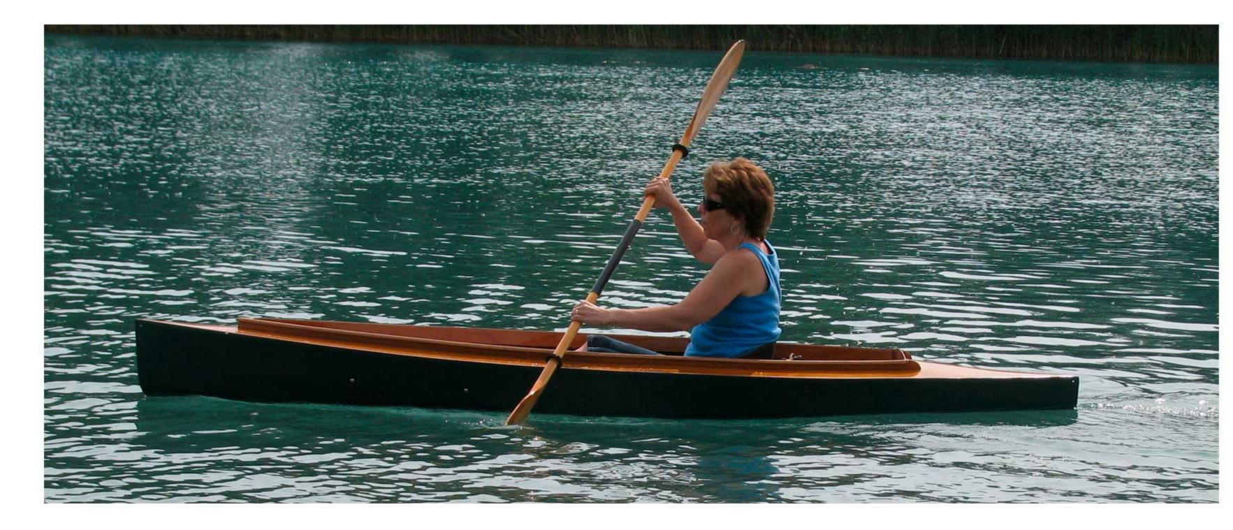
Length 10 ft. 3.05 m. Beam 26 in. 66 cm. WL Beam 24 3/8 in. 62 cm Weight\* 34 lbs. 15.4 kg. Recommended Load Range 120 to 175 lbs. 54 to 80 kg.
