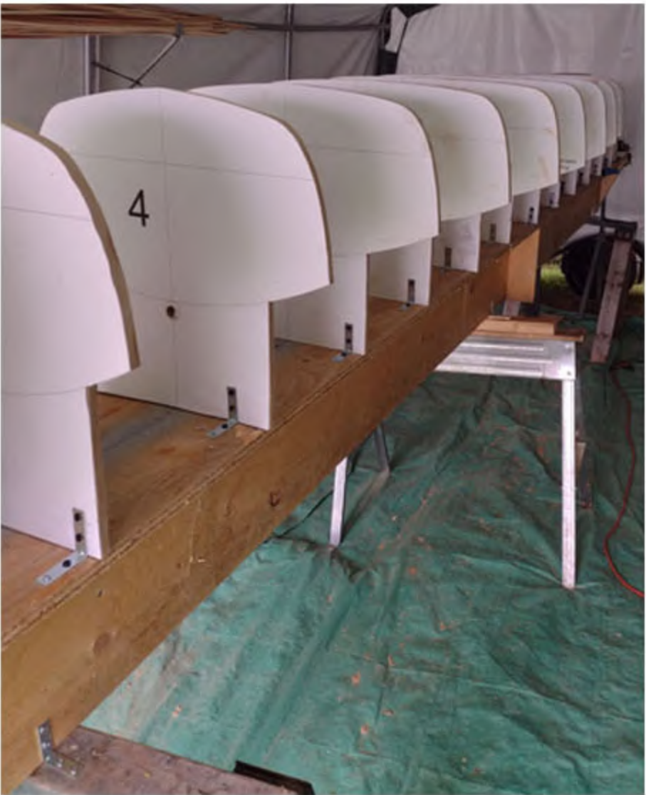
Molds set up for construction of a Pukaskwa 20. Photo: RHW
